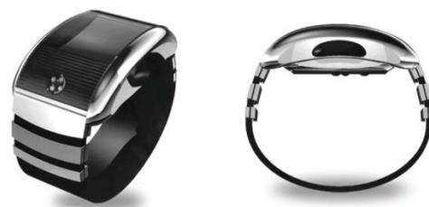
Figure 2: Health watch prototype developed at CSEM for the monitoring of motion related and cardiac activity parameters.
