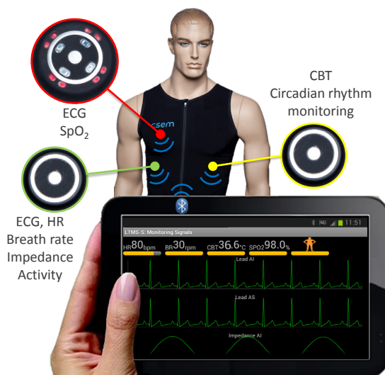
Figure 1: Overview of LTMS-S monitoring capabilities.
