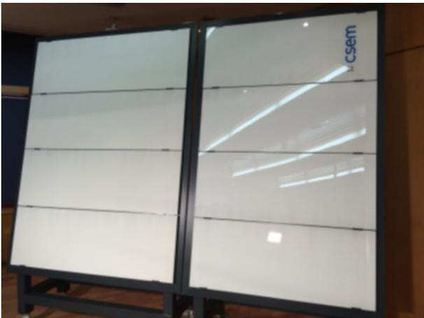
Figure 1: White PV modules fabricated at CSEM.
