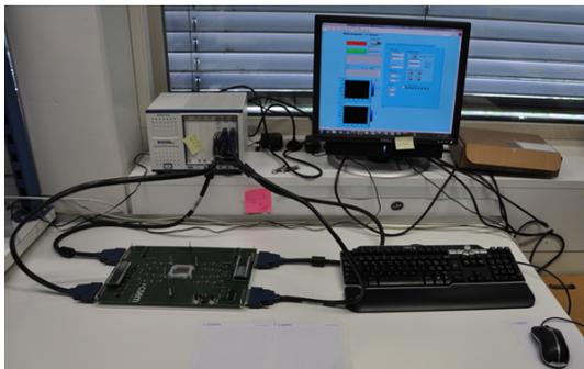
Figure 2: CSEM's multi-purpose bi-directional PC interface platform.
