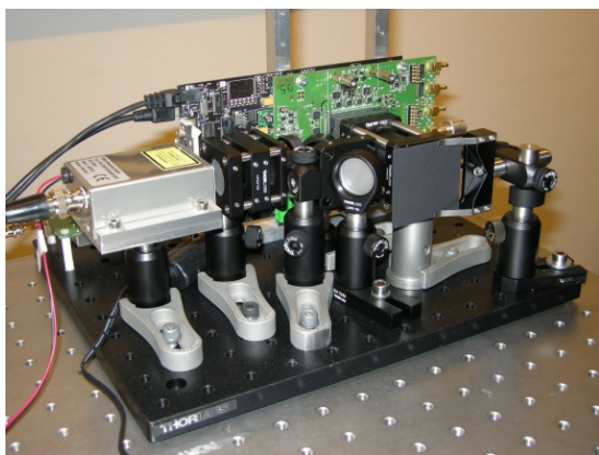
Figure 1: Optical setup for wide-field FLIM, allowing a 2D map of fluorescence lifetimes with nanosecond resolution.
