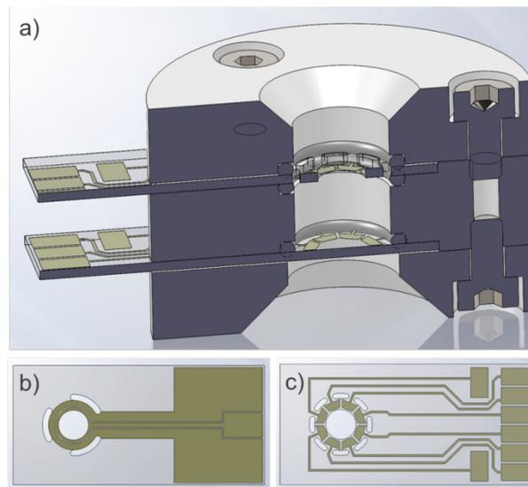
Figure 2: a) Cross-section of biochamber with integrated electrodes; b) Design with 2 electrodes (for one side); c) Design with six electrodes (for one side).
