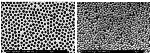
Figure 1: SEM pictures of structures of 500 nm large holes (left) and 100 nm pillars (right).
