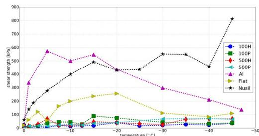
Figure 2: Dependence of adhesion strength on temperature between 0 and  $-50\text{ }^{\circ}\text{C}$ . 100/500=structure size in nm; H=holes, P=pillars.
