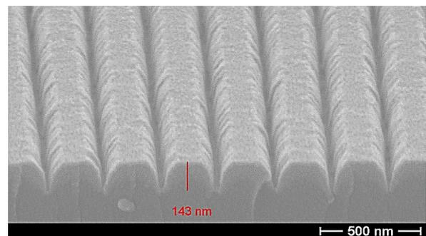
Figure 3: SEM cross-section of a  $\text{Ta}_2\text{O}_5$  subwavelength grating manufactured by RIBE, hard masking and lift-off. The original top interface of the layer is left intact, enabling a low roughness making it suitable for being bonded.
