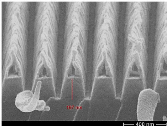
Figure 1: Cross-section image using SEM of a subwavelength grating etched by RIBE in  $\text{Ta}_2\text{O}_5$  after nano-imprint resist removal by solvent. A massive material re-deposition can be observed on the ridges.
