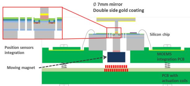
Figure 1: 2D tilting electromagnetic deflecting mirror concept.
