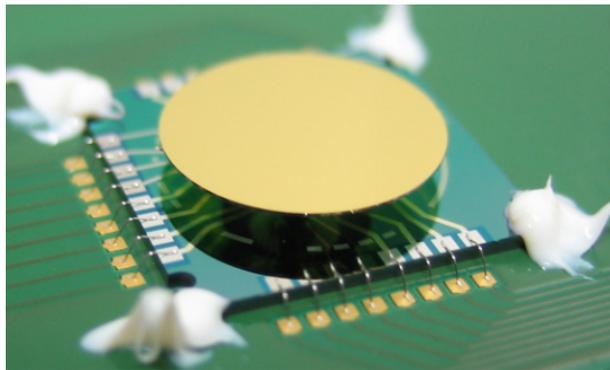
Figure 2: Assembled MEMS scanner with integrated position sensors.
