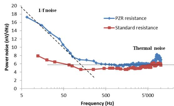
Figure 3: Noise level of a piezoresistor bridge.
