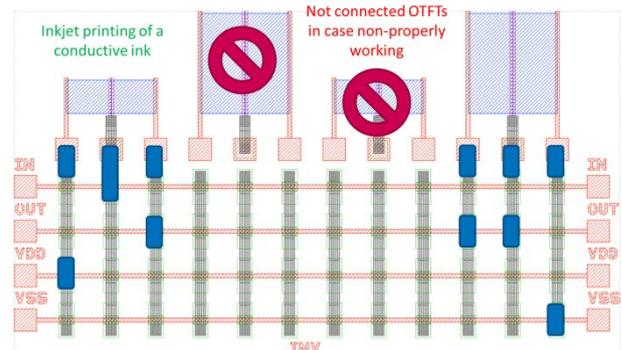
Figure 3: Inkjet Gate Array approach illustrated on Zero-Vgs Inverter.
