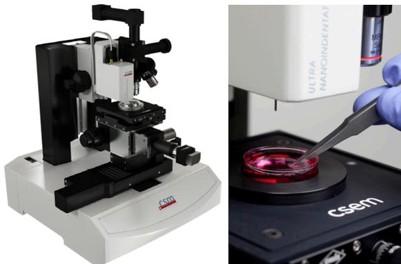
© CSEM / CSM Instruments – *The Bioindenter is a new instrument dedicated for the mechanical analysis of soft biological samples in physiological conditions.*
