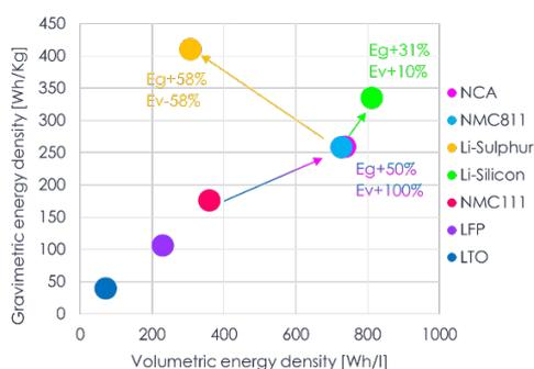
Figure 1: Chemistries' positioning as regards energy densities.
