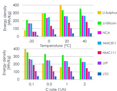
Figure 2: Dependence of energy density of various chemistries on current and temperature.
