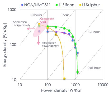
Figure 3: Ragone chart of tested technologies vs. application.
