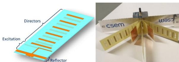
Figure 1: Antenna element model (left) and realized sectorial antenna (right).
