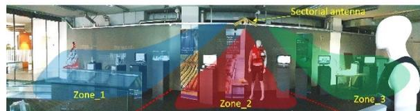
Figure 3: Sectorial antenna indoor test @ CSEM showroom.
