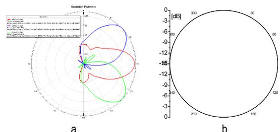
Figure 2: Antenna radiation pattern comparison (@2.45 GHz): HFSS simulation (a) and measured (b).
