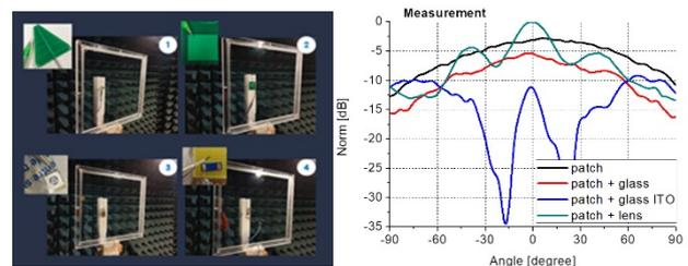
Figure 2: Window antenna characterization with different source antennas (left) and normalized measured antenna gain (right).
