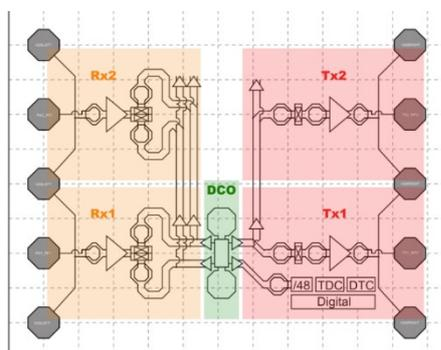
Figure 1: Block diagram of the core.
