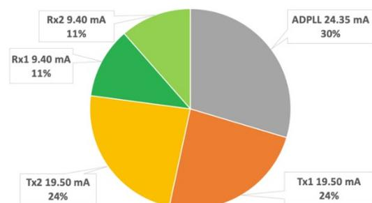
Figure 3: Current consumptions with 0.8 V voltage supply.
