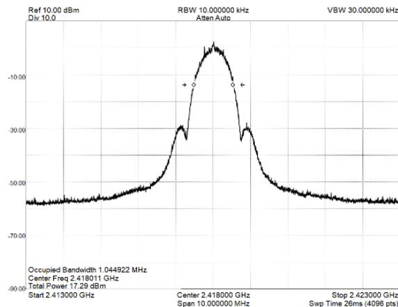
Figure 2: Tx GFSK modulation spectrum.
