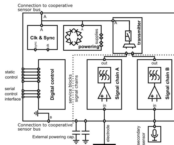
Figure 2: Block diagram of the cooperative-sensing IC.
