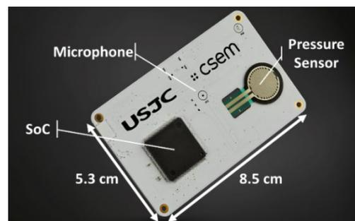
Figure 2: Demonstration board (credit card format).
