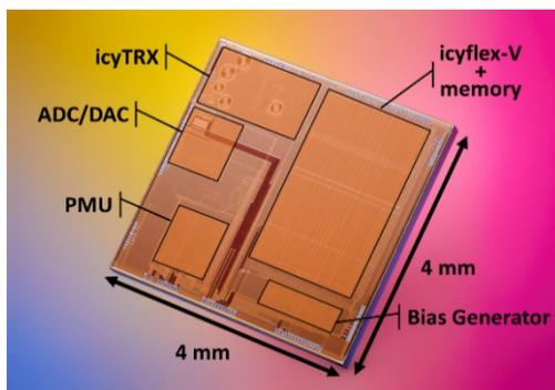
Figure 1: SoC microphotograph.
