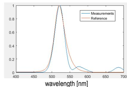
Figure 3: Miniature photo-spectrometer measurement of a green LED, exact spectrum (reference, in red) and measured spectrum (in blue).
