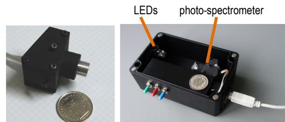
Figure 2: The fabricated miniature photo-spectrometer (left), a suitable housing including LEDs and USB connector (right).
