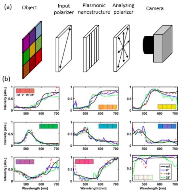
Figure 1: a) Plasmonic nanostructures used as tunable filters for imaging; b) Reconstruction of color spectra from colored patches (Machbeth ColorChecker) recorded with a conventional spectrometer (ref.) and the imaging system at tilt angles of 0, 15, and  $25^\circ$ .
