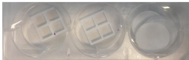
Figure 3: SLA printed structures from a barium titanate NP based composite resin.
