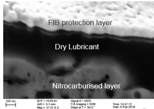
Figure 1: Focused Ion Beam (FIB) section showing the continuous interface between the lubricant and the nitrocarburised layer.
