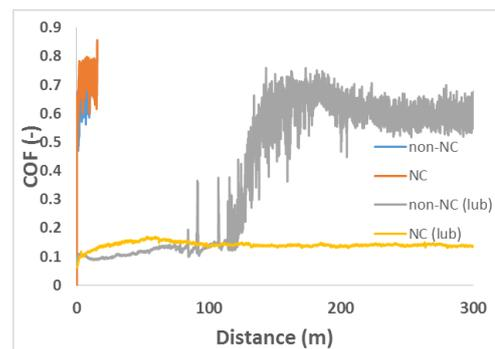
Figure 2: COF evolution (applied force =0.5 N) on non-impregnated NC and non-impregnated non-NC, as well as impregnated NC steel (hybrid surface) compared to impregnated non-NC (reference surface), showing the advantage of the hybrid surface.
