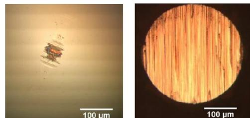
Figure 3: Optical microscope images of the 2 mm diameter steel counter body (load 0.5 N) after 400 m of sliding on the hybrid surface (NC, left) versus the lubricated reference surface (non-NC, right). The hybrid surface reduces drastically the wear of the steel counterpiece.
