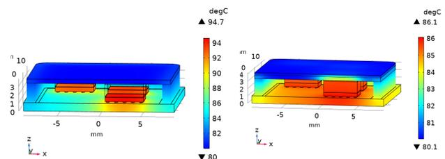
Figure 2: Temperature plot of chips dissipating 1 W each in flip-chip mount. Right: chip backside additionally connected to lid (SiC/Cu-D spacer + Ag paste).
