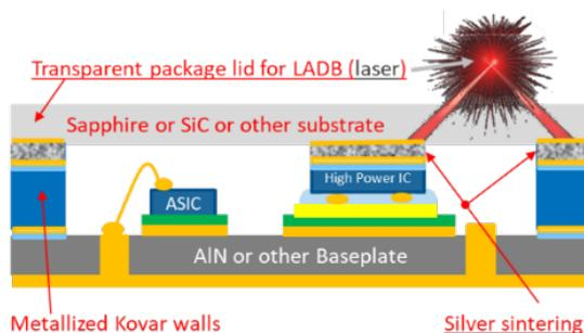
Figure 1: LADB (laser) hermetic sealing and back-side chip bonding on the lid to efficiently remove heat with silver paste sintering.
