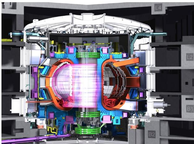
Figure 1: Schematic view of ITER tokamak.
