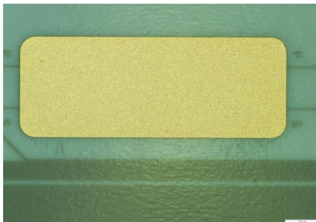
Figure 2: Detail of absorber with electrical contact lines seen through the thin substrate.
