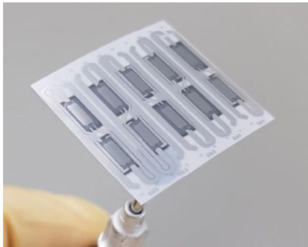
Figure 2: 5-channel bolometer sensor ( $25 \times 22 \times 0.02 \text{ mm}^3$ ).
