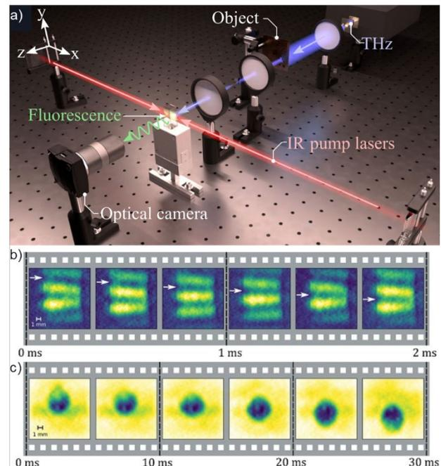
Figure 3: Fast 2D THz imaging demonstration by the University of Durham. a) lab setup, b) chopper wheel imaged at 3'000 frames per second, and c) falling water drop imaged at 500 frames per second.
