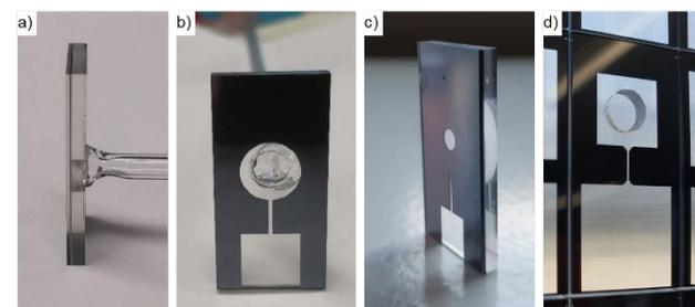
Figure 2: MEMS atomic vapor cell fabricated at the wafer-level for: a,b): gas sensing (with a stem attached by the University of Stuttgart), c): GHz sensing and imaging and d): THz imaging.
