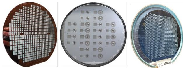
Figure 1: MEMS atomic vapor cell fabricated at the wafer-level for: OPM (left), GHz/THz (middle), and MAC (right) applications.
