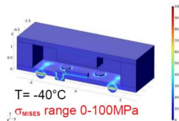
Figure 5: Example of Von Mises stress-plot for comparative analysis of adhesive choices at  $-40^{\circ}\text{C}$  during thermo-cycling test.
