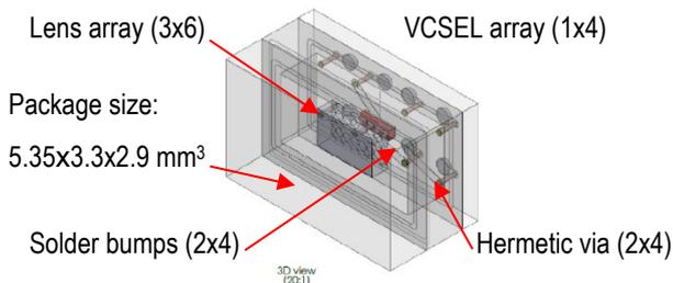
Figure 2: Parametric CAD Model including focusing lens (Solidworks).
