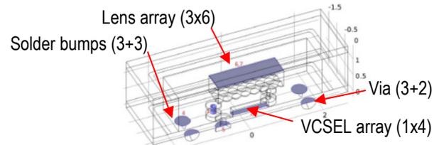
Figure 4: FEM model imported and cut to half-symmetric (COMSOL).
