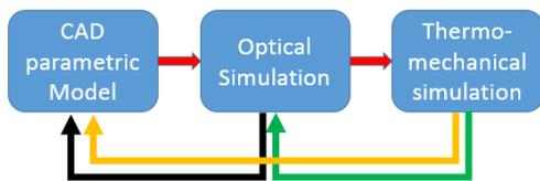
Figure 1: Optical micro-packages design flow.
