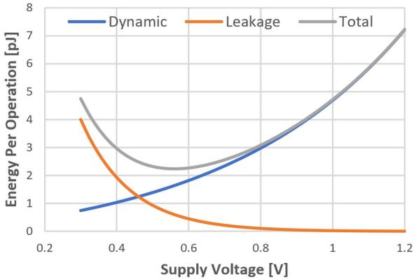
The Minimum Energy Point (MEP) is for most CMOS processes in the sub-threshold or near-threshold region. The challenge is that in this region the process variation also has a much bigger influence, and therefore most digital designs have been done with higher voltages.
