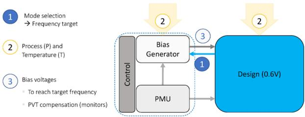
CSEM's Adaptive body biasing and frequency scaling IP and design methodologies make it possible to design digital blocks with just the same robustness as for conventional designs, but with the benefits mentioned above.
