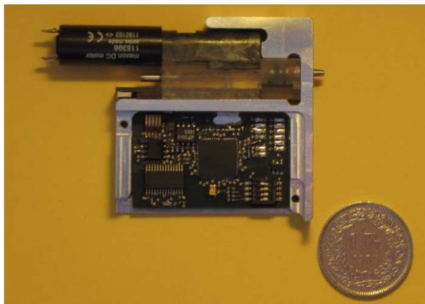
Figure 1: Turbisc pump with an integrated flow sensor and closed-loop control electronics utilizing CAN interface for communication.
