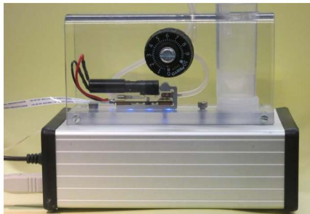
Figure 3: Demonstrator of the Turbisc pump with an integrated flow-sensor. An arbitrary flow resistance can be set with the dial.
