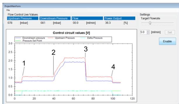
Figure 2: Constant flowrate run of the closed-loop Turbisc pump. Red and blue represent the upstream and downstream pressure of the flow restriction, the set point for pressure difference is displayed in green and the measured pressure difference in magenta.
