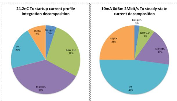
Figure 2: Transmitter start-up and steady state currents
