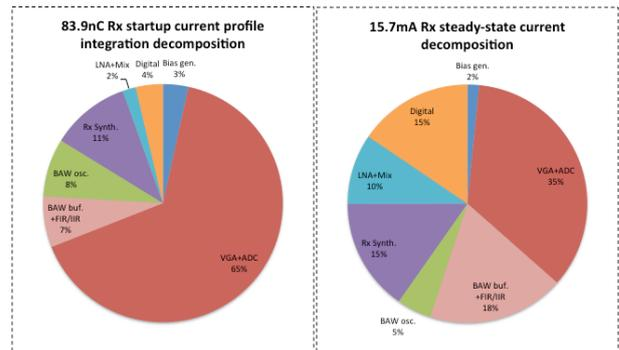
Figure 3: Receiver start-up and steady state currents
