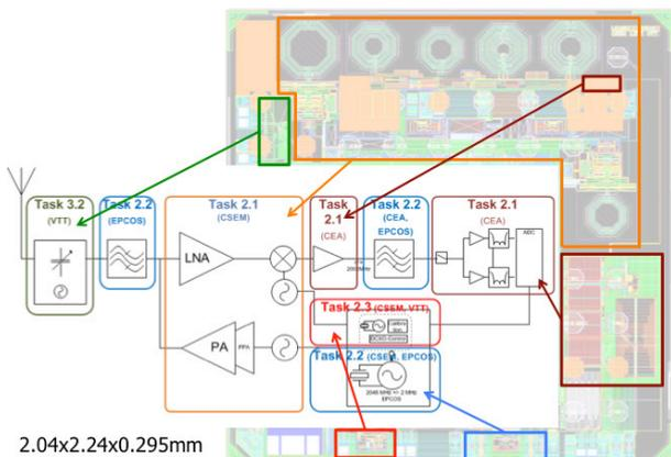
Figure 1: Radio transceiver architecture and associated layout
