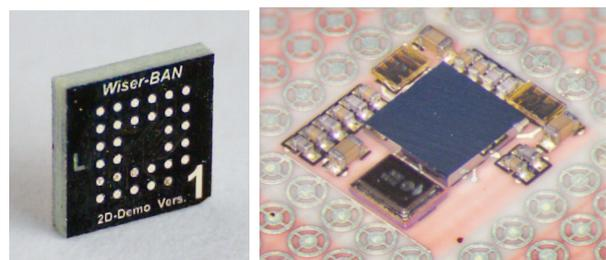
Figure 4: 4.25 x 4.25 x 0.77 mm system-in-package
