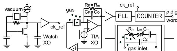
Figure 2: Simplified block diagram of the gas density read-out circuit.
