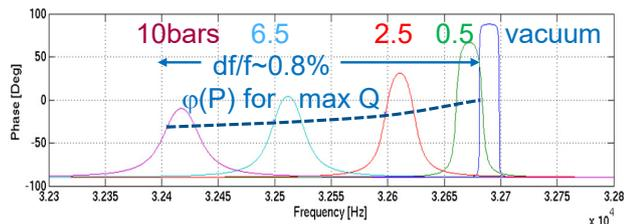
Figure 1: Measured phase of a 32 kHz XTAL at various SF<sub>6</sub> pressures.
