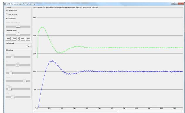
Figure 3: Example Python GUI for motor speed PID control.
