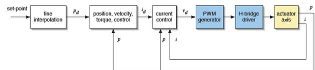
Figure 2: Closed-loop motor control block diagram.
