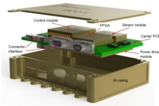
Figure 1: Conceptual view of the MCC-X assembly.
