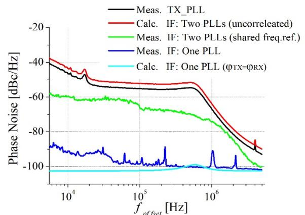
Figure 1: Calculated and measured values of the correlated phase noise.
