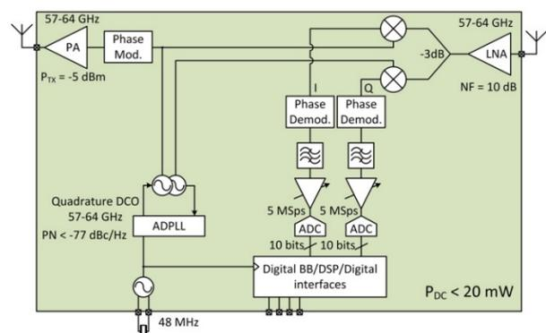
Figure 2: Block diagram of the RADAR architecture.
