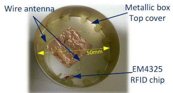
Figure 2: RFID tag and wire antennas location in the metallic box (top cover).
