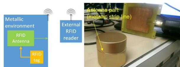
Figure 3: Block diagram of the RFID in the metallic box solution and implemented solution under laboratory test.
