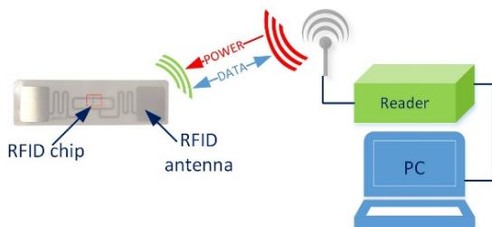
Figure 1: Basic RFID communication system blocks.
