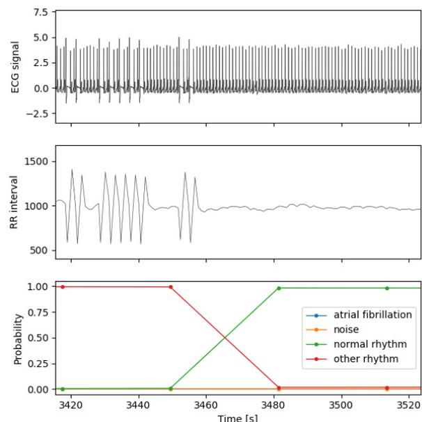
*Figure 1: Cardiac rhythm classification from an ECG signal recorded with the smart vest. The ECG signal (top) includes premature ventricular contractions which are visible in the RR intervals (middle). The NN correctly identifies this segment of the signal as reflected by the class probabilities (bottom).*
