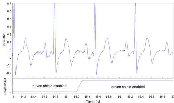
Figure 2: EMI resilience before and after activation of the driven shield.
