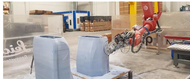
Figure 2: The KRAKEN robot machining the Pininfarina car mock-up.
