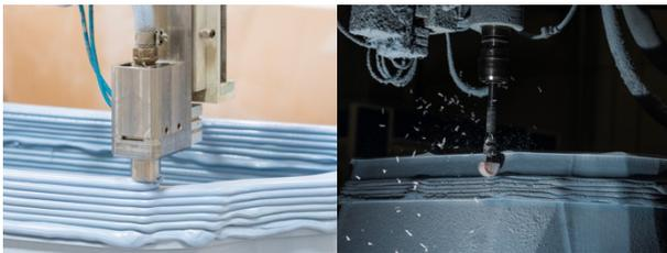
Figure 1: Climb-up HM process, (left) Resin AM; (right) Milling.
