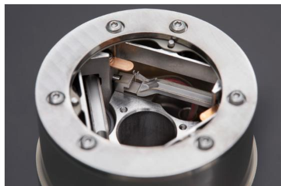
Figure 3: CLUPI CFM detailed view of the flexures.
