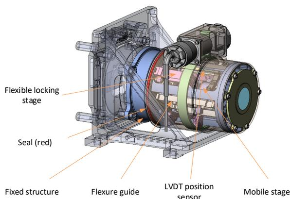
Figure 2: CFM (CLUPI Focus Mechanism) building blocks.
