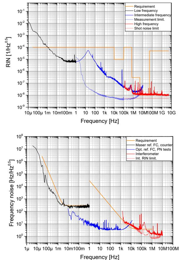
Figure 2: Top Relative intensity noise (RIN) and bottom frequency noise of the CSEM laser breadboard. The orange lines represent the required specifications.
