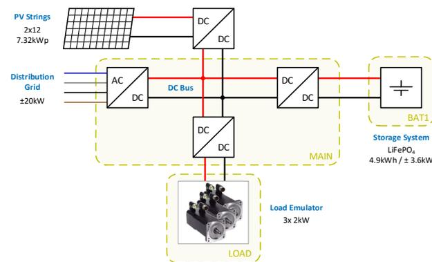
Figure 1: General topology of the microgrid.
