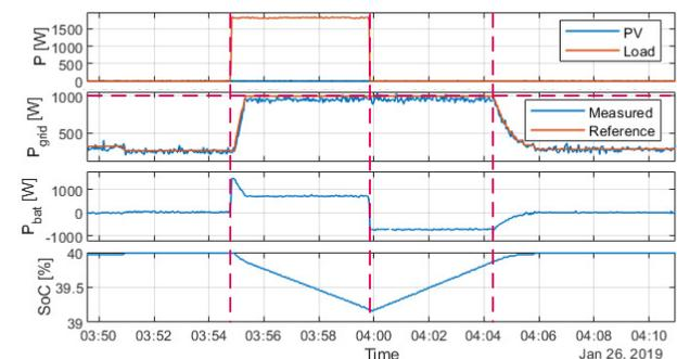
Figure 3: Load, PV, grid and battery power profiles and evolution of battery state of charge during a peak-shaving event.
