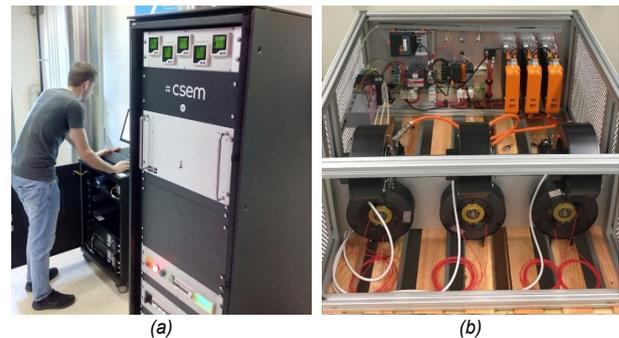
Figure 2: Main and battery cabinet (a) and load emulator (b).
