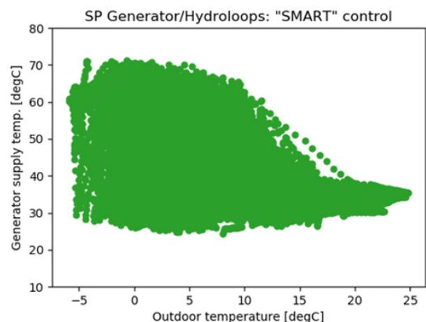
Figure 2: Flow temperature distribution of central heating unit.
