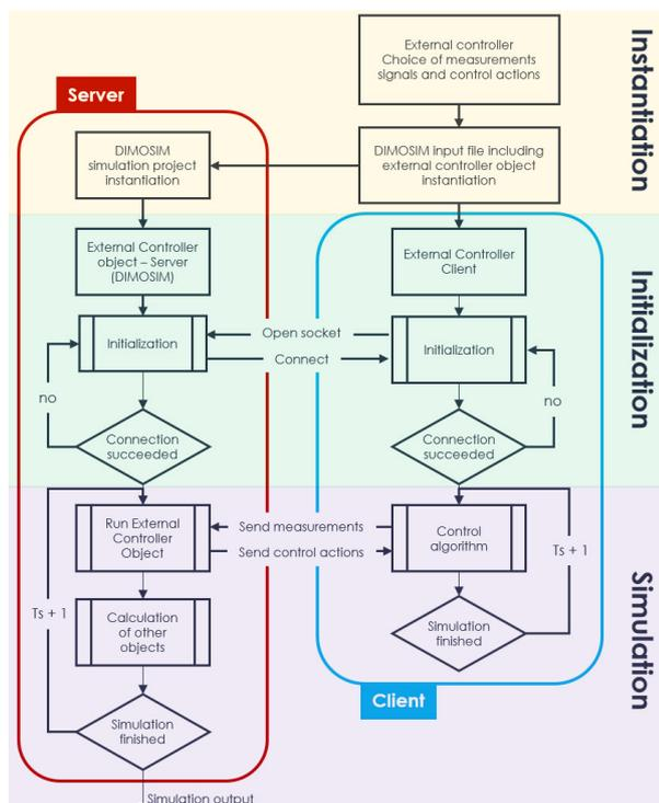
Figure 1: Interaction of building simulator and optimization algorithm.
