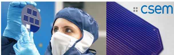
Figure 1: Illustration of test structures used to first achieve 24.2% certified efficiency on 4 cm<sup>2</sup> solar cells early 2019 using all CSEM processes, transferred to industrial silicon wafers.
