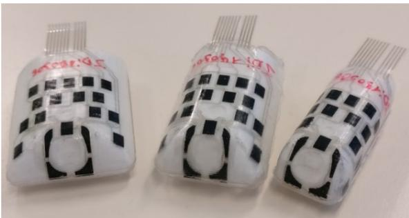
Figure 1: Pressure sensors for robotic grippers (F&P Robotic case).
