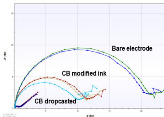
Figure 1: Nyquist plots of the EIS analysis of the different SPEs using 1 mM  $[\text{Fe}(\text{CN})_6]^{3-/4-}$  in 0.1 M KCl solution as redox probe.
