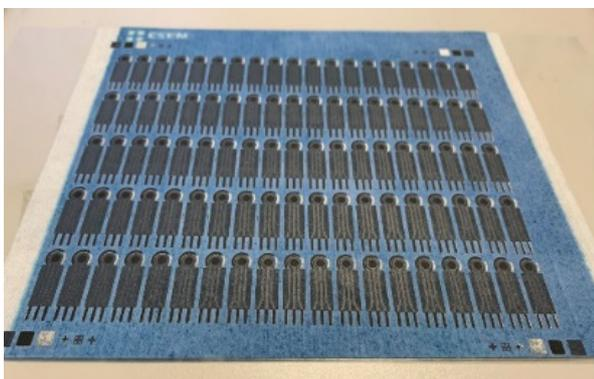
Figure 1: pH sensors printed on a cotton substrate.
