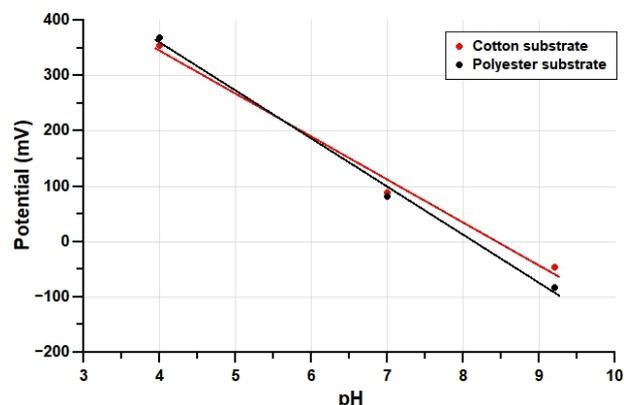
Figure 2: Response at 3 different pH (4.01-7.00-9.18) made by using pH sensors printed both on cotton and polyester.
