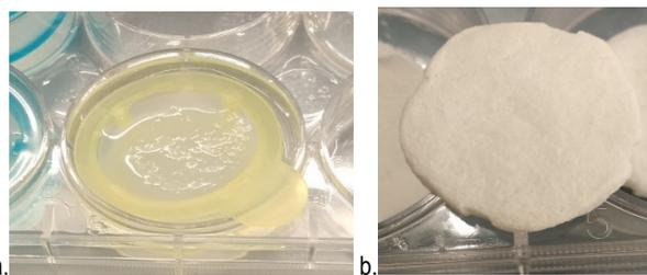
Figure 3: (a) Mixing of the nanofibrils and reagents for cross-linking; (b) Finished nanocellulose scaffold.
