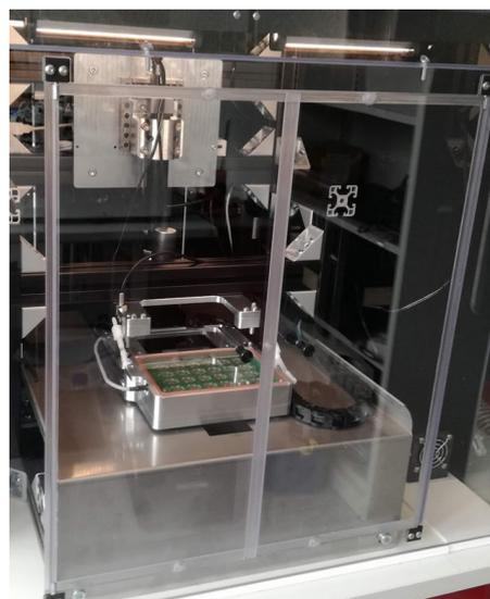
Figure 3: Automated force measurement system for 3D printed muscle tissues developed by the partners of the ongoing InnoSuisse project.
