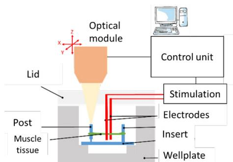
Figure 2: Schematic representation of automated force measurement system based on well-plate inserts that translates the muscles force into post displacement.
