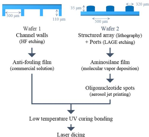
Figure 1: Fabrication process of the microfluidic microarray device.
