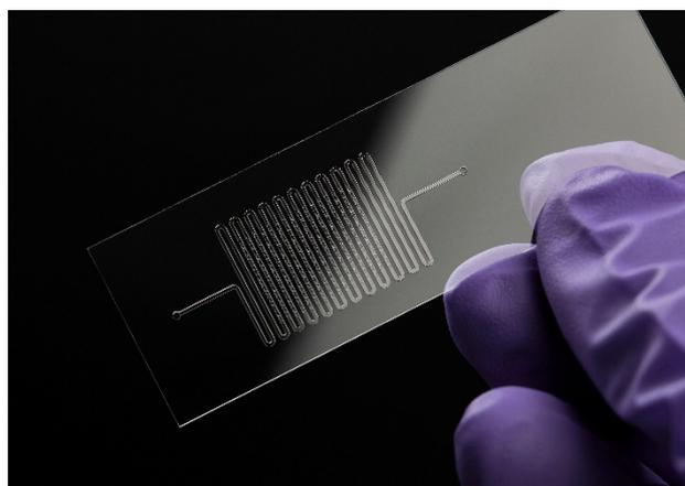
Figure 2: Picture of the sealed glass microfluidic microarray device.
