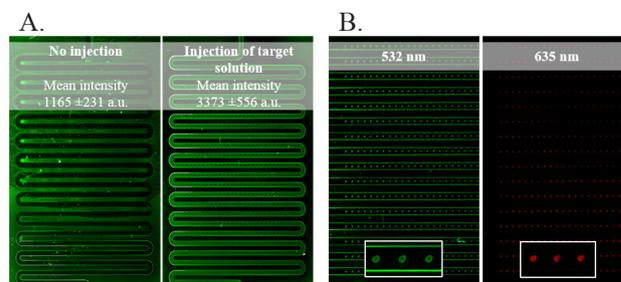
Figure 3: Example of fluorescence images obtained before and after injection of a fluorescent solution in the channel, 4 months after sealing (A) and results obtained after bonding and hybridization of the pre-immobilized target (B).
