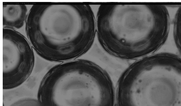
Figure 3: Optical images of monodisperse PLGA encapsulated oil in water emulsion prior to solvent evaporation and conversion to solid PLGA microspheres.
