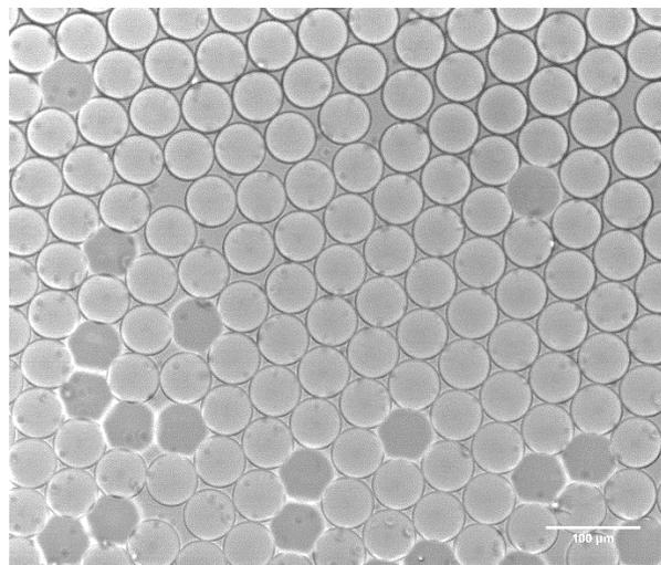
Figure 2: Highly monodisperse water in oil droplets generated with membrane emulsification device, droplet size around 50 μm (droplet size is tunable with nozzle geometry).
