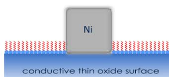
Figure 1: Schematics showing self-assembled monolayers (SAMs) used as a masking layer for electroplating of nickel, then copper on thin conductive oxides.
