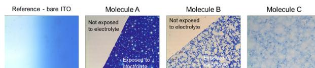
Figure 3: Microscopic images of the etched ITO after 10 minutes dipping in a highly acidic electroplating solution.
