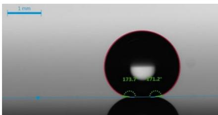
Figure 2: Water droplet behavior on pyramid-textured ITO surfaces.
