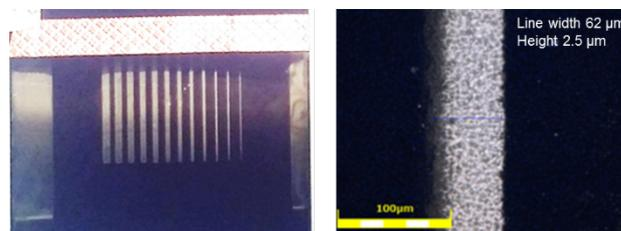
Figure 4: (left) Picture of sample after nickel electroplating using a SAM as resist; (right) Scanning confocal microscopy image taken on the thinnest line of picture shown left.
