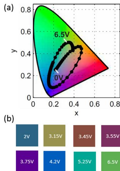
Figure 2: (a) CIE plot of color range spanned by the system. White: colors obtained by mechanical rotation of an analyzing polarizer. Black: colors obtained by increasing the voltage applied to the liquid crystal cell from 0 V to 6.5 V. (b) Colors at particular voltages.
