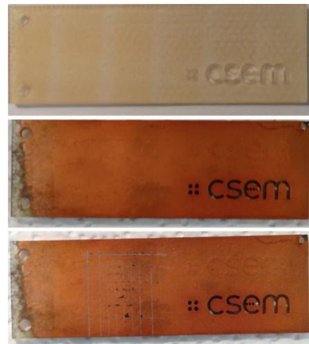
Figure 2: (top) 3D printed plastic sample by stereolithography (SLA); (middle) the same sample after the metallization process; (bottom) the same sample after the adhesion test.
