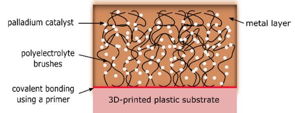
Figure 1: Surface preparation by covalent binding of polyelectrolytes onto 3D-printed plastics and subsequent metallization by electroless plating.
