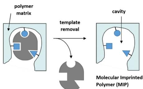
Figure 1: Principle of MIP detection.
