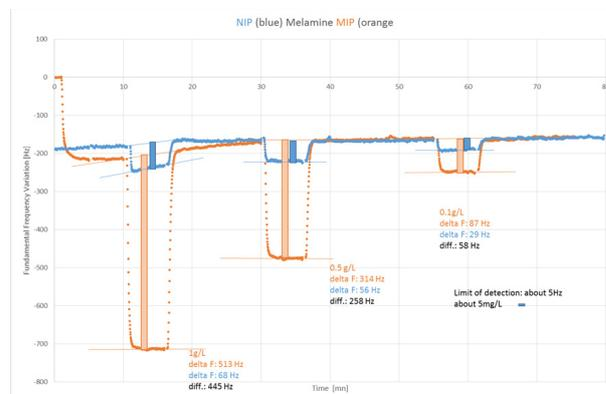
Figure 2: Melamine detection for a MIP deposited on QCM. The curve with the smaller amplitude corresponds to the NIP (Non-Imprinted Polymer).
