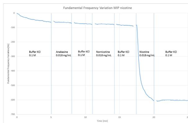
Figure 3: MIP detection of nicotine on QCM. Comparison with the signal obtained with anabasine and nornicotine.
